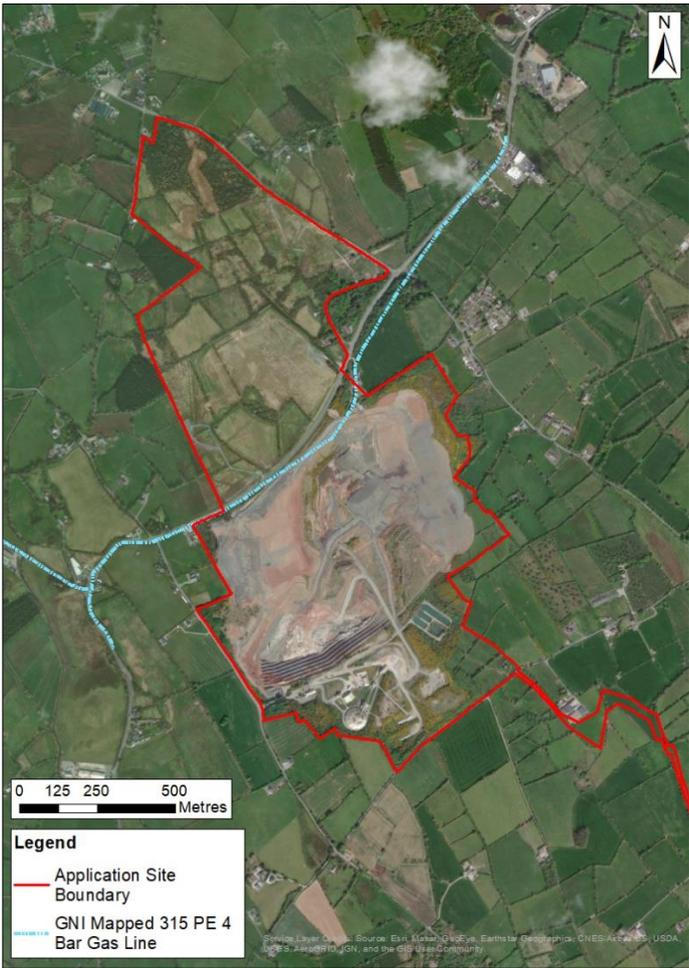
Figure 16.3: Gas service plan redrawn from GNI supplied maps
